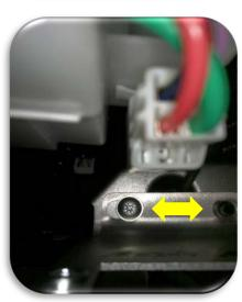
mount bracket on plastic tab an fix it with the previously removed screw (magnetic screwdriver required)
