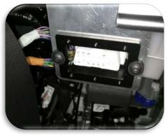
mount both (housing and socket jack) onto the mounting bracket with the provided fillister screws
