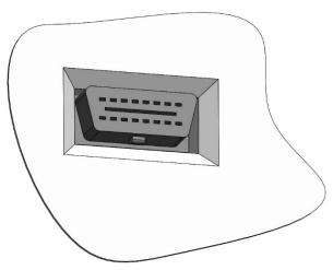
remove the original OBD socket jack from it's housing
